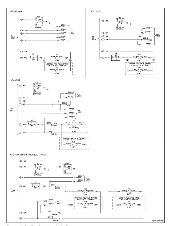
Figure 3-10 Gas Fuel Connections Wiring Diagram
